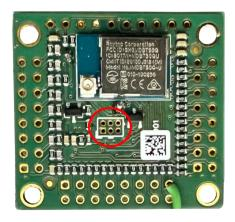
• Connect the external antenna to the antenna connector (marked on the picture below); without an antenna, the range of the Kit is greatly decreased.
