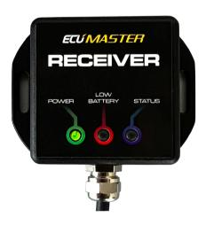
**Green LED:** Glows indicating the Wireless Receiver is powered. If properly powered, the diode should glow constantly.
